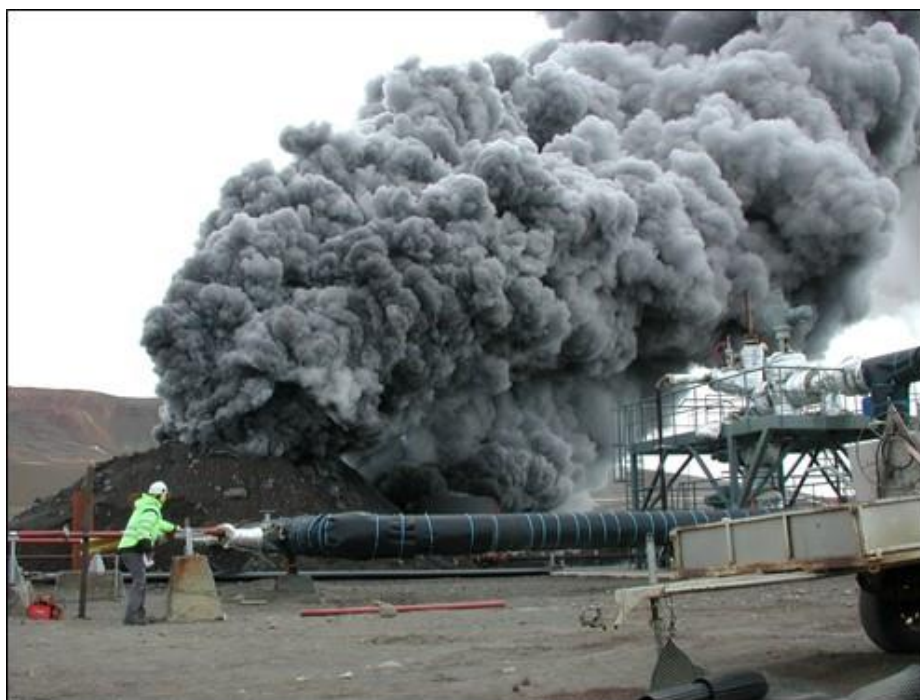
Figure 17. The beginning of a flow test of IDDP-1 (photo G. Ó. Friðleifsson).
