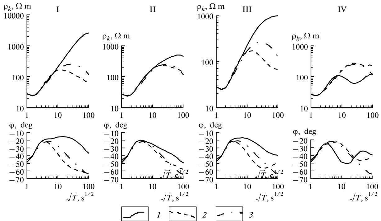
**Fig. 6.** Typical MTS curves for the regions in Fig. 5. Roman numerals are the numbers of the typical curves corresponding to the regions in Fig. 5. 1, 2, and 3 are the transverse, the longitudinal, and the locally normal MTS curves.
