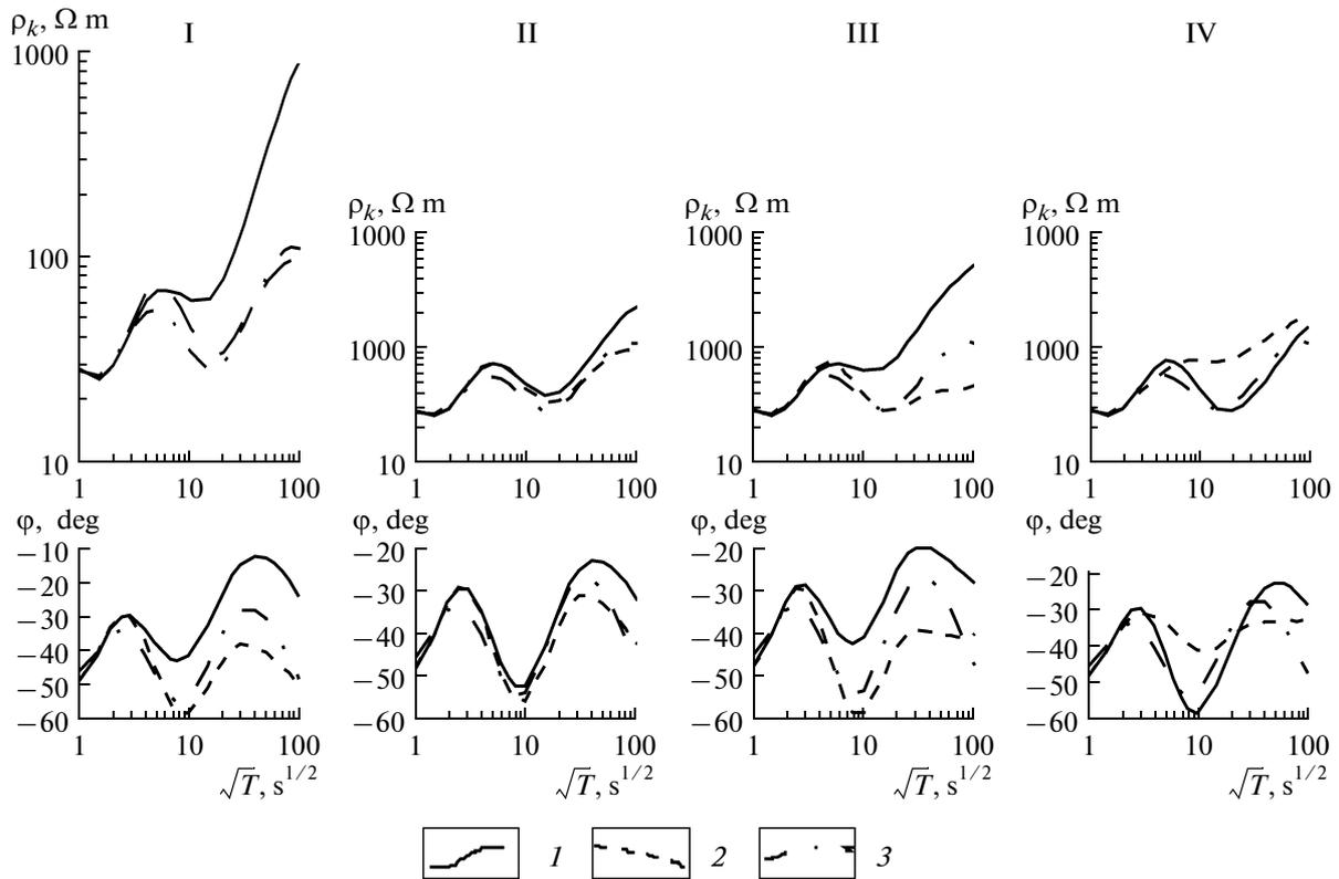
Fig. 7. Typical MTS curves in the model of Kamchatka containing a crustal conductive layer. Roman numerals are the numbers of typical curves corresponding to the regions in Fig. 5. 1, 2, and 3 are the transverse, the longitudinal, and the locally normal MTS curves.
