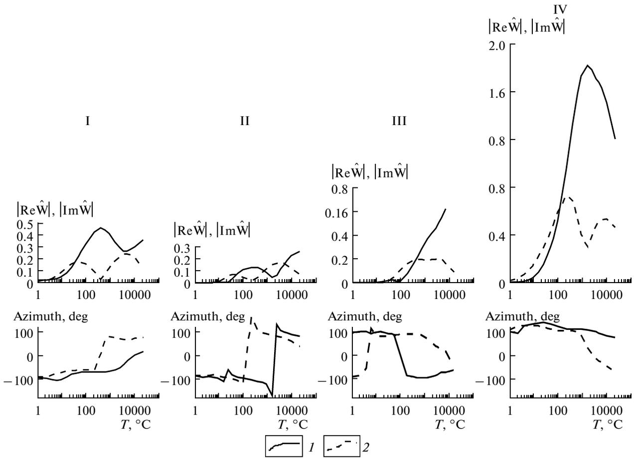
Fig. 3. Typical frequency curves of the magnetic tipper for the zones in Fig. 2: @1 and @2 the curves of the magnitudes and the azimuths of the real and imaginary induction arrows.
