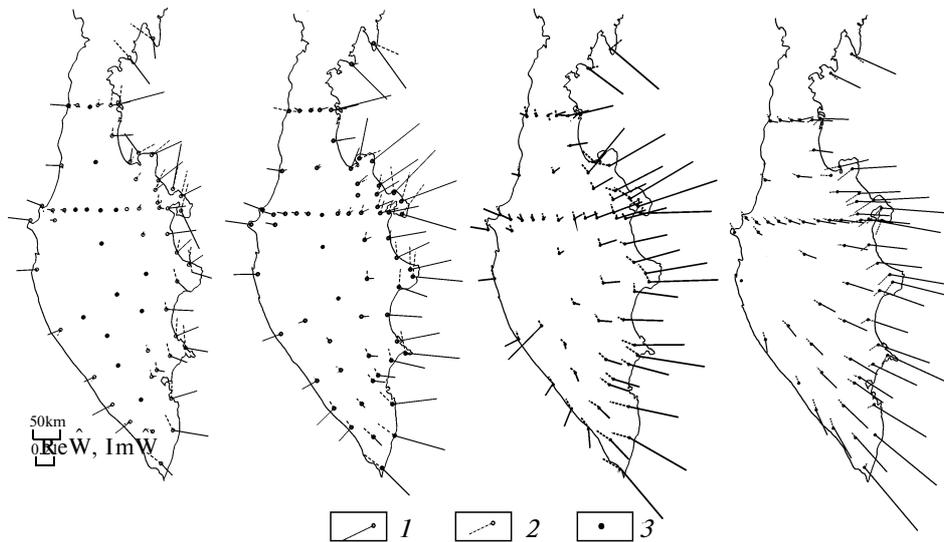
**Fig. 4.** The behavior of the induction arrows at the periods (a) 100 s, (b) 400 s, (c) 1600 s, and (d) 10000 s: 1 and 2 the real and the imaginary induction arrows, respectively; 3 the sites where the vectors are close to zero.
