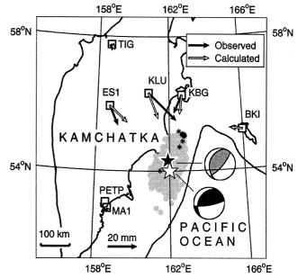
Figure 6. Post-seismic motions after the Kronotskoye earthquake and their fit from their inversion for a deviatoric moment tensor point source. The assumed location of the model source is within the aftershock area at a depth of 30 km (white star); its focal mechanism is shown by the black and white beachball. The source is equivalent to an  $M_w = 7.9$  event. The observed and calculated vectors at station BKI are practically identical. For other notation see the caption to Fig. 4.
