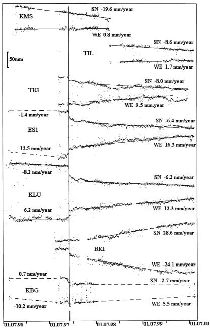
Figure 2. Displacements of seven Kamchatka stations with respect to station PETP along the N and E directions for 1996–2000 and estimates of average velocities. The vertical line depicts the time of occurrence of the  $M_w$ =7.8 Kronotskoye earthquake of 1997 December 5.
