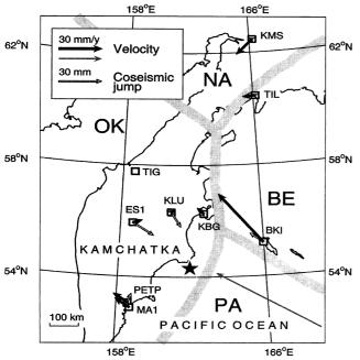
Figure 1. Average velocities of GPS stations (squares) for 1998–2000 and coseismic jumps caused by the major Kronotskoe earthquake of 1997 December 5,  $M_w$ =7.8. Station TIG is assumed to be fixed. Grey arrow depicts the velocity of the assumed rigid Pacific plate. Black star indicates the location of the Harvard CMT centroid of the major event. Plates are as follows: PA, Pacific; NA, North American; OK, Okhotsk; BE, Beringia.
